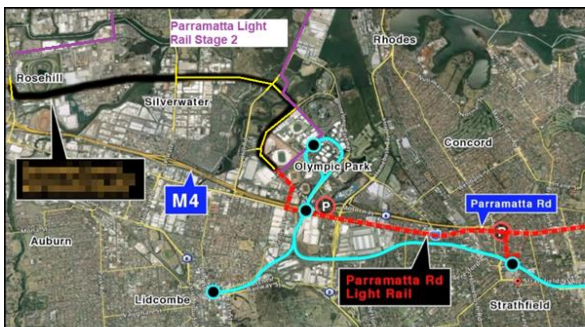
Fig 6. The proposed Parramatta Road Light Rail to meet the Parramatta Light Rail Stage 2 at Carter St
